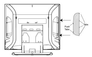
Figure 3. Replacing Input Cover
